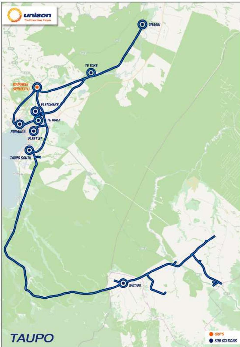
Figure 2 – Taupo GXP's and Substations
